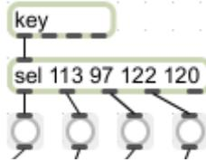
*The sel object routing out the signal, when keys Q,A,X and Z is pressed.*
