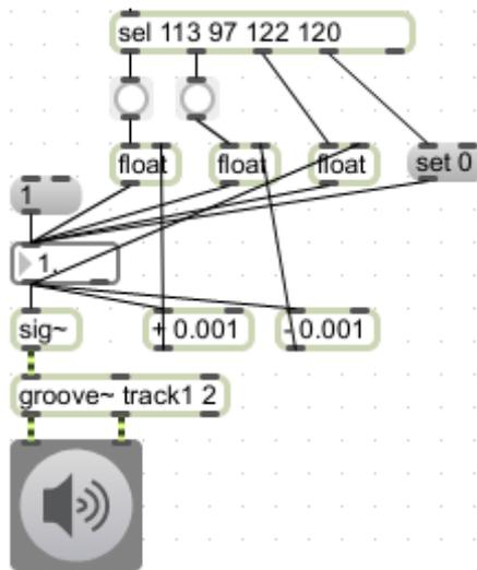
Basically all we need to do now, is duplicate the patch and make sure that our key input is different for this one, and that our buffer~ and groove~ objects are named track2 2 in their extension instead of track1.
